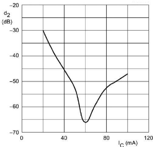
$V_{CE} = 12 \text{ V}; V_o = 316 \text{ mV}; f_{(p+q)} = 810 \text{ MHz.}$
