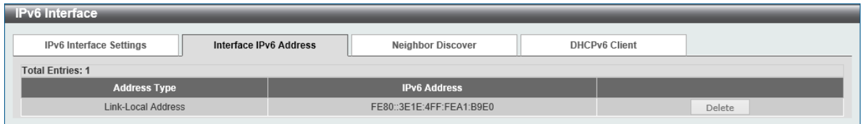
Figure 6-15 IPv6 Interface - Detail, Interface IPv6 Address window
