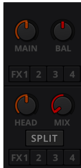
Fig. 21: The headphone and main mix knobs
