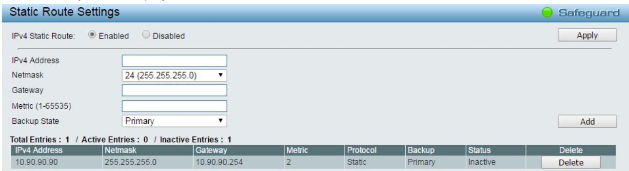
Figure 4.101 – L3 Functions > IPv4 Static Route – Static Route Table
