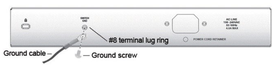
Figure 2.10 – Connect a Grounding Cable
